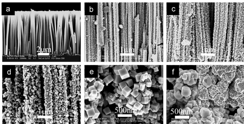
Fig. 1. SEM images of Si NWs (a), Si NWs/Cu<sub>2</sub>O nano-heterojunction with different deposition time: 2 min (b), 5 min (c), 10 min (d) and morphology with 10 min deposition time at different pH value: pH=12.5 (e) and pH=13 (f).
