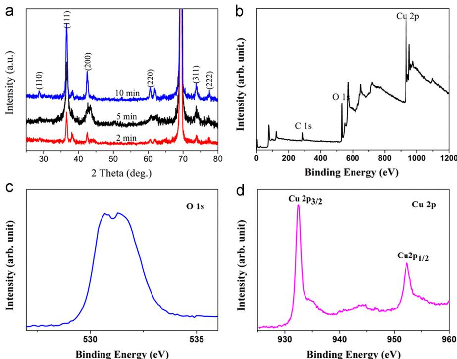
Fig. 2. XRD patterns ((a)) and typical XPS spectrum ((b)–(d)) of Si NWs/Cu<sub>2</sub>O nano-heterojunction.
