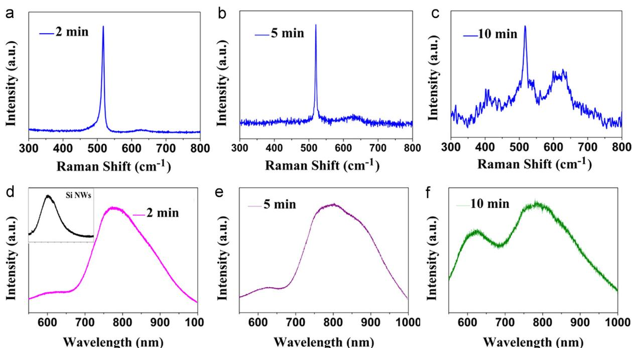
Fig. 3. Raman and PL spectra of Si NWs/Cu<sub>2</sub>O nano-heterojunction with different deposition time of Cu<sub>2</sub>O.
